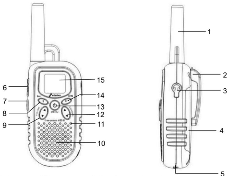
**1 Antenna** (The antenna is fixed to the housing, do not try to unscrew it!)
