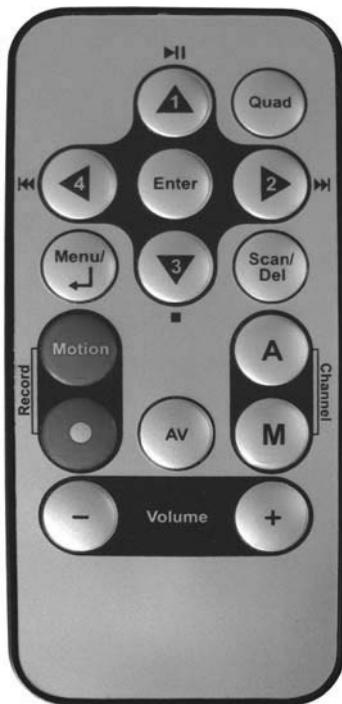
If motion is detected by the camera(s), the monitor will beep and display the image from the triggered camera. The monitor will return to scan mode about 5 seconds after the alarm has completed. Press **Scan**, **(Channel) A** or **(Channel) M** buttons will cancel scan mode.
