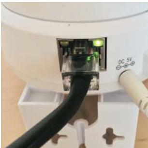
The green LED flashes. After approx. 15 seconds, the yellow LED lights up. The connection between camera and router is connected.
