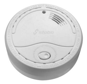
The photoelectric cell installed in the stabo smoke alarm device checks the ambient air for smoke particles which occur in the event of a fire. Both an optical (rapidly flashing LED) and an acoustic (piezosiren 85 dB (A)/3m) alarm is triggered if a certain smoke particle concentration is reached.
