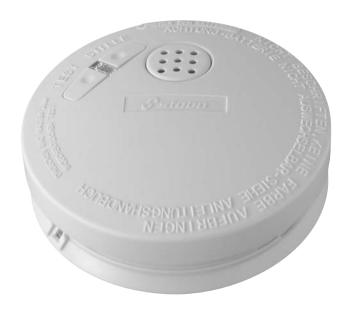
The photoelectric cell installed in the stabo smoke detector checks the ambient air for smoke particles which occur in the event of a fire. Both an optical (rapidly flashing LED) and an acoustic (piezosiren 85 dB (A)/3m) alarm is triggered if a certain smoke particle concentration is reached.
