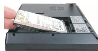
Position the hard disk at an angle (connections facing to the front side) in front of the hard disk slot. Now push the hard disk inwards and downwards for inserting the connector strip (1) into the slot (2).
