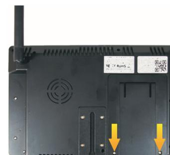
Undo both screws from the cover of the hard disk compartment and remove the cover.
