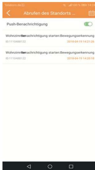
Use the calendar function to view the motion alarms triggered on the last days. Tap the **calendar icon**. Set the day now and tap **Bestätigen** (Confirm). A list containing the number of currently triggered motion alarms plus the date and time is shown.
