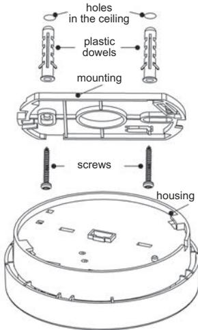
Mark the position for the drilling holes at the mounting position by using the mounting as a drilling jig.
